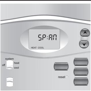
3. Span setting mode – allows you to adjust the system ON/OFF cycle rate. The default setting is 2 (the system cycles ON or OFF when the temperature is within 1° F (0.5° C) above and below the set temperature.) The span setting can be adjusted if your system is cycling too fast or too slowly.
